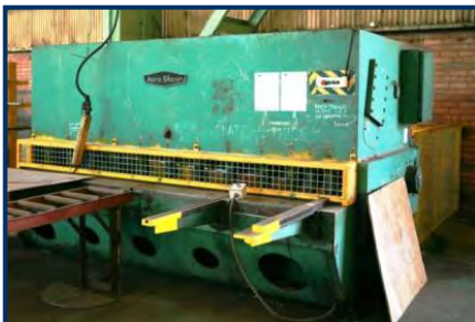
Plate guillotine 3100mm wide x 16mm thick
