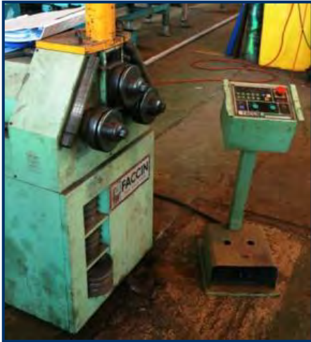
Horizontal and Vertical Section Rolls, Capacity – 100 x 100mm Angle, 100mm Flat Bar & 180NB pipe
