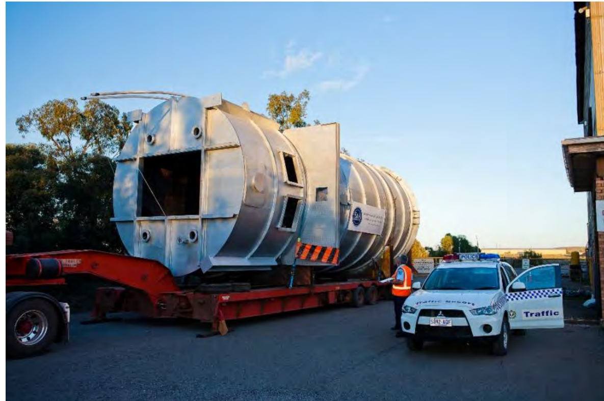
16m x 4.5m Vertical Kiln for Penrice
